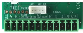
All low voltage connections are made with a 12 pin pluggable connector. Just above the connector is the 6 pin **FTDI** connection for uploading new firmware and accessing the command line interface (CLI).
