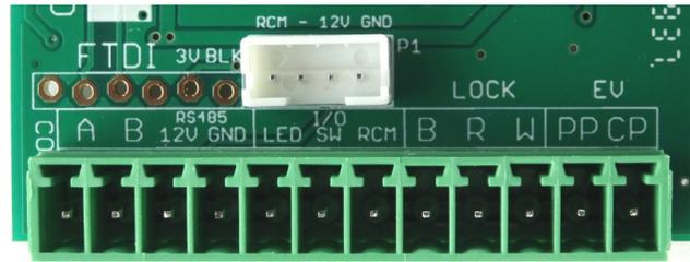
All low voltage connections are made with a 12 pin pluggable connector. Just above the connector is the 6 pin **FTDI** connection for uploading new firmware and accessing the command line interface (CLI).
